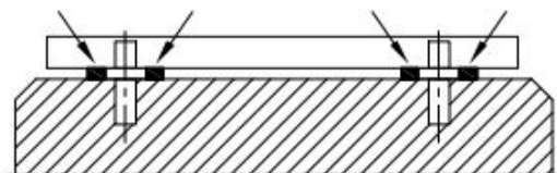
Fig. 2. Foundation, baseplate and fitting the shims
